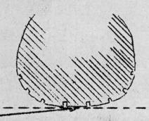
When there is very little thread area in contact with the road surface, the front end will be very sensitive and have a tendency to weave, particularly when riding on straight roads.
