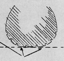
The tires in which the recommended air pressures are maintained will handle well at all speeds on straightaways and turns. Therefore it is IMPORTANT that you check your tire prssures at least every 200 miles.
